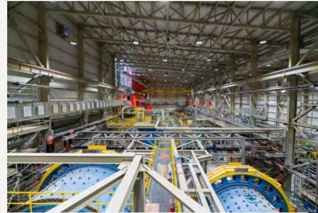
Process Plant – Comminution Circuit
